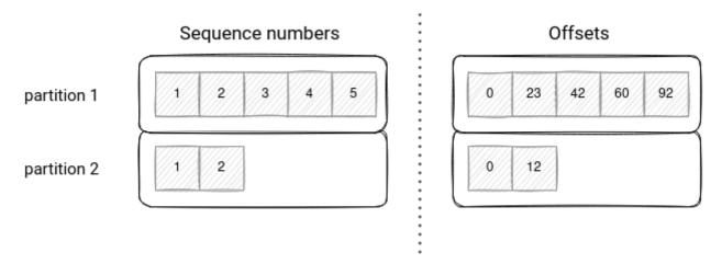
On the other hand, the sequence number is a continuous number of the event within the partition. It increases by 1 whenever the broker appends a new event to the partition. For the reprocessing scenario it should be easier to reason about the sequence numbers than the offset numbers.
